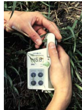
Figure 3. Use of SPAD meter to assess N sufficiency.
